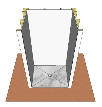
Engineered panels are cut, drilled and siliconed to the Drywall.
