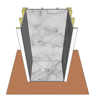
After the shower panels are installed, the curb and trim are installed around the bottom perimeter.
