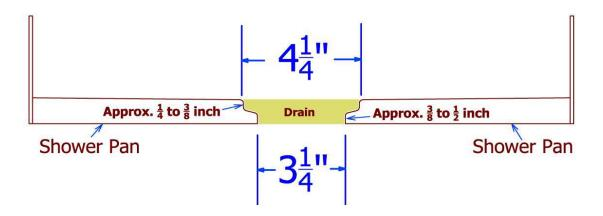
Substrate material (sheet rock, etc.) should not be installed until after the plumber has connected the plumbing to the pan. The substrate material (drywall/ Denshield) should stop about one inch above the flange of the pan.
